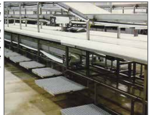
Photo on Right: FGI-AM ® grating was utilized for work station platforms that could adjust to the height of the line workers.
